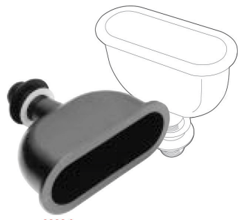
6023 Anti-syphon bottle trap Adjustable height neck - requires adaptor 6009, 6012 or 6013 to connect to pipework.
